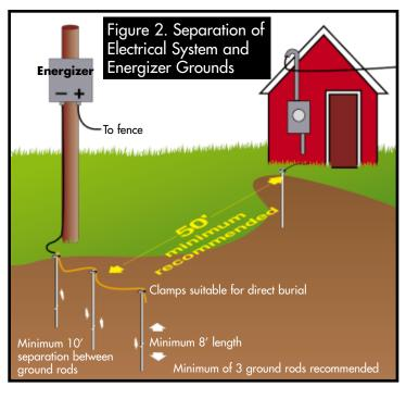
**lead cable** (20,000 volt insulation is recommended). Electrical wire of the type used for the building wiring, with 600 volt insulation, must never be used for this purpose.
