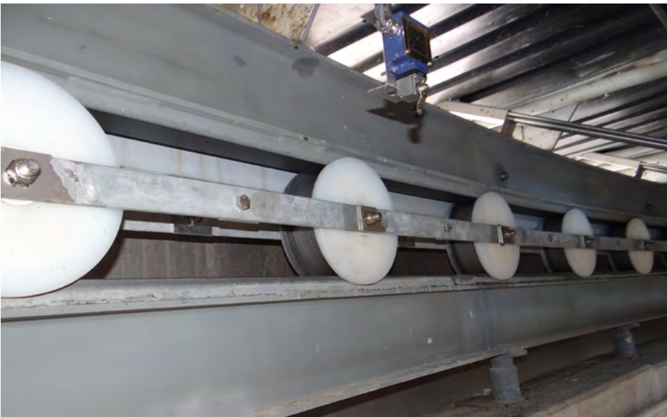
Self-tracking patented nylon multiroller system
