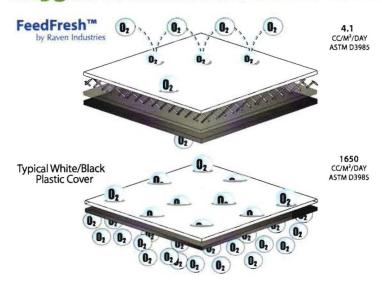
400 Times Less Oxygen (0₂) Passes Through FeedFresh™ Silage Covers
