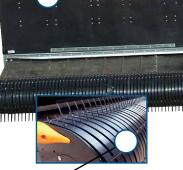
Center cam drive: Strong support, minimal gap between heads
