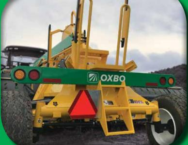
**NEW!** Rear mounted hydraulic tank and access platform make hydraulic system maintenance easier
