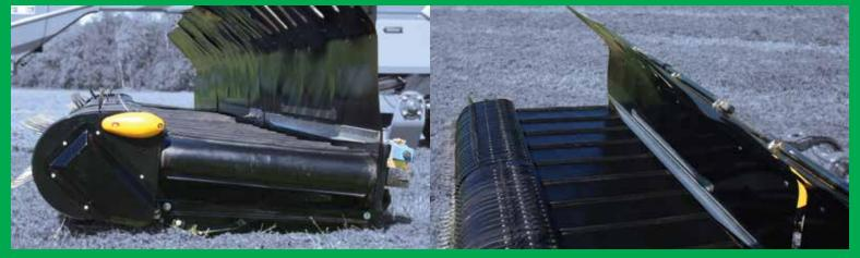
NEW! Wide 40" conveyor with a rear profiled slope. More room for heavier crop and the 5° angle distribute the crop more evenly for a better windrow
