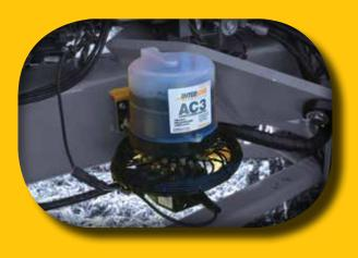
NEW! Quick access allows you to fill or monitor OPTIONAL auto-lube
