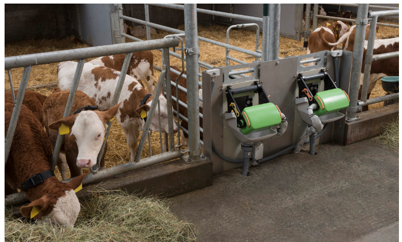
Supplying feed to CalfRail and groups using only one automatic feeder
