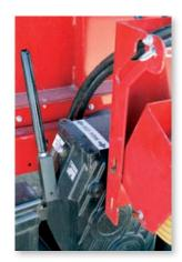
Two speed PTO driven gearbox for slow speed mixing and high RPM for better cleanout. Optional hydraulic shifter allows shifting from the cab of the tractor.
