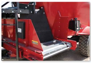
Side Discharge or Front Center Flat Sliding Conveyor Feeds Out of Either Side - Optional Fixed or Adjustable Incline Conveyors to match your feeding needs.
